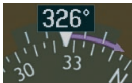
Figure 3.4.17 Turn Rate Indicator and Trend Vector
